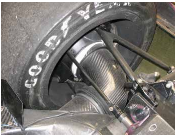
The high downforce nature of the US circuits in 1992 highlighted the Jaguar's weakness - wheel failure at Lime Rock led to a large accident
